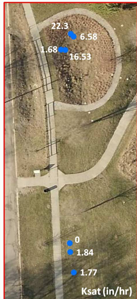
Figure 16. K_{sat} measurement locations and values at Orchard Park. Note that NULL values are represented as zero (0).
