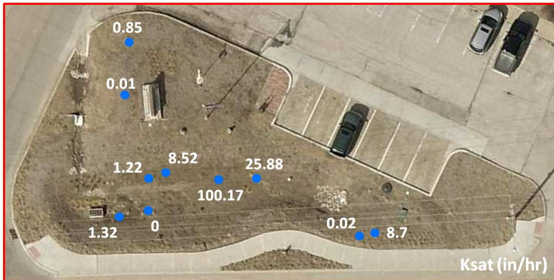
Figure 22. K_{sat} measurement locations and values at the Omaha Sewer Maintenance Facility. Note that NULL values are represented as zero (0).
